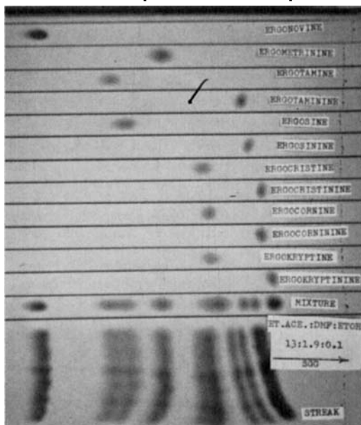
Fig. 1.—Thin-layer chromatogram of mixture of ergot alkaloids. (Solvent system A .)
