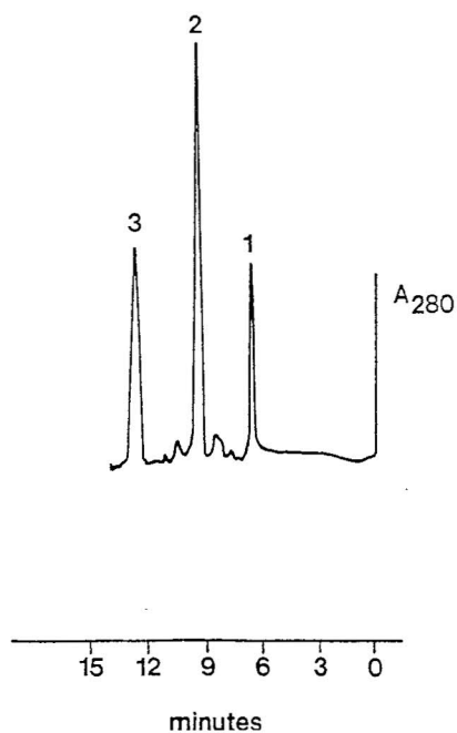
Figure 1. Reversed-phase liquid chromatographic separation of N,N-disubstituted MDA derivatives. Peaks: 1 = N-methyl-N-ethyl MDA; 2 = N-methyl-N-i-propyl MDA; 3 = N-methyl-N-n-propyl MDA.
